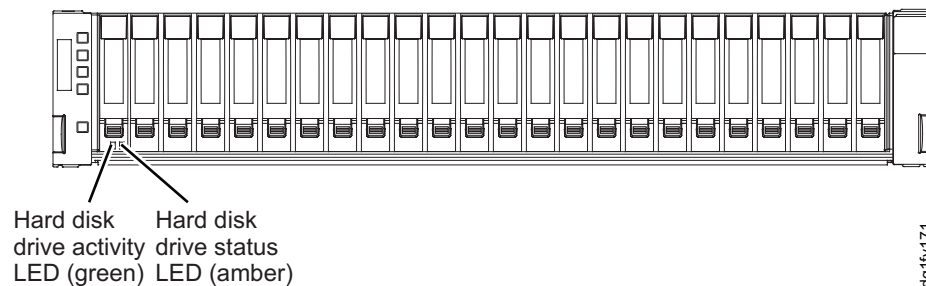
Figure 99. DS3524 storage subsystem and EXP3524 storage enclosure drive LEDs
